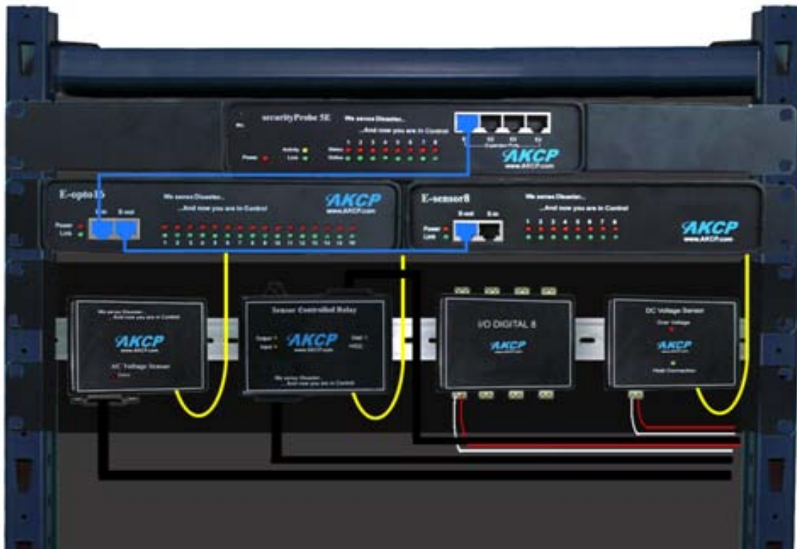
Example concept mounting AKCP devices and sensors using the rack mount kit system
